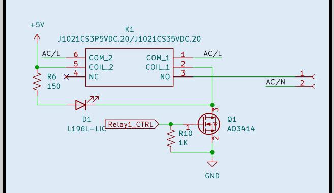
Our current implementation of the relay sub system involves use of MOSFETS to provide the relays with the current they need for operation.
