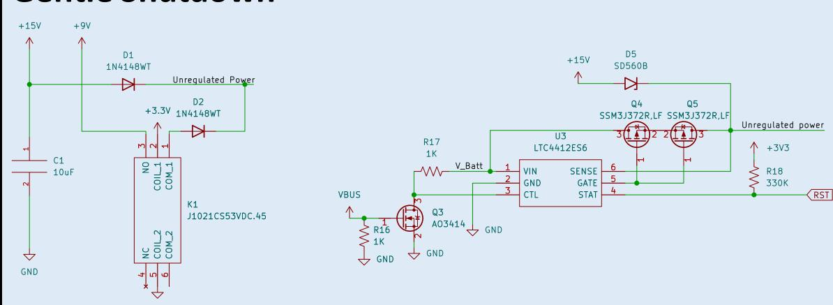
If 5V rail drops from the BBB after shutdown begins, the OS will corrupt. This was our first attempt fixing this using a 9V battery which discharged into the 5V regulator if the 15V rail was shut off. The final revision utilizes a LIPO battery charging circuit (not pictured) in tandem with the 5V regulator to provide the BBB with 5V when the 15V rail is down. We use MOSFETs to alternate where the BBB sources 5V.
